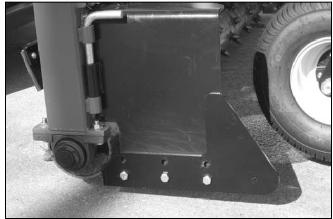
Side Shield shown with optional Side Shield Extension in down position.
